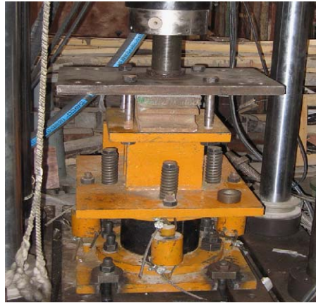
Fig. 1. Multidimensional earthquake isolation and mitigation device.
