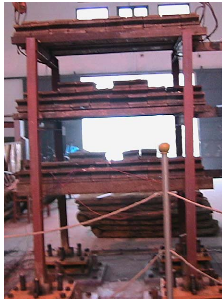
Fig. 4. Shaking table tests on the structure.
