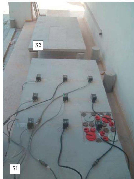
Fig. 5. Reinforced concrete slabs and measurement equipment.
