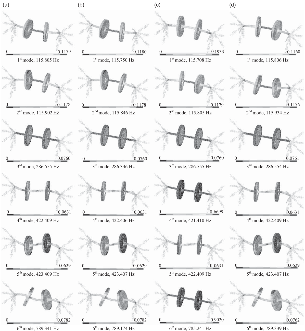
Fig. 2. Numerically generated mode shapes and natural frequencies (modes 1–6) for (a) a healthy shaft, (b) a cracked shaft, (c) combined misalignment, and (d) a bent shaft.
