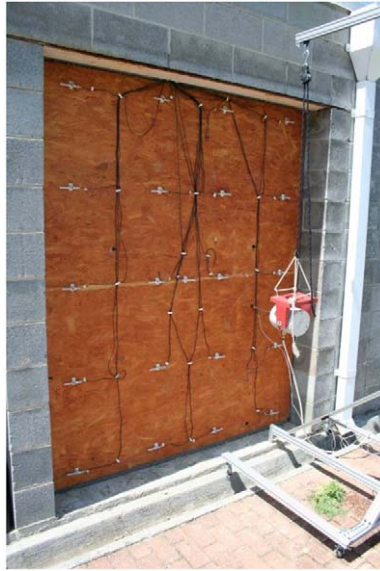
Fig. 23. Experimental setup of the modal test.
