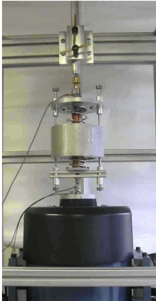
Fig. 3. Testing of the 2-DOF mechanical analogue on the electrodynamic shaker.
