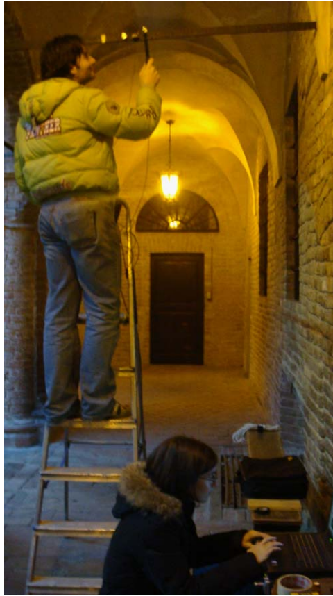
Fig. 4. Experimental measurement on tie-rod “1”.
