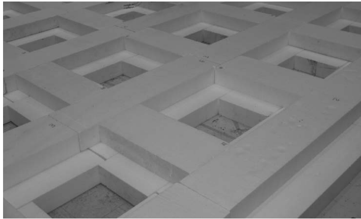
Fig. 13. The studied 2D periodic profile with two waveguides—Profile A.
