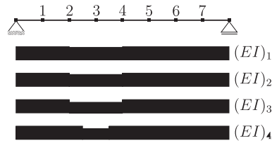
Fig. 6. Damaged simply supported beam: measurement points and EI distribution for all four damage scenarios.
