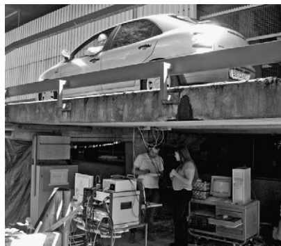
Fig. 5. The reinforced concrete bridge ramp tested at the University of Stuttgart, Germany.
