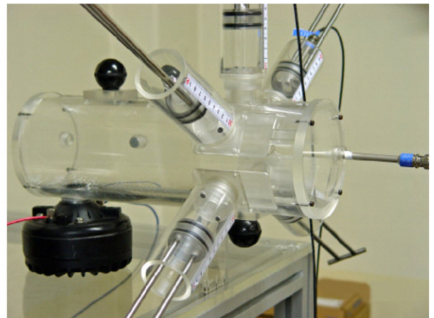
Fig. 2. Schematic of a model chamber and adopted acoustic cavities.
