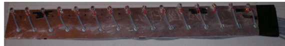
Fig. 11. A photograph of the in-duct microphone array. Fifteen 7 mm electret microphones were mounted on a thin 50 mm by 400 mm aluminium plate. The microphones were positioned at the edge of the plate, with the centre of the capsules 25 mm apart.
