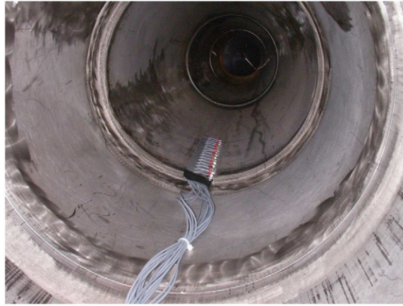
Fig. 12. A photograph of the microphone array positioned in the duct. The microphones themselves lay on an axial line, and are as close as possible to the duct wall.
