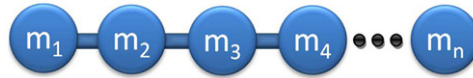
Fig. 1. Schematic of a filter based on n resonators coupled in an open-chain configuration.
