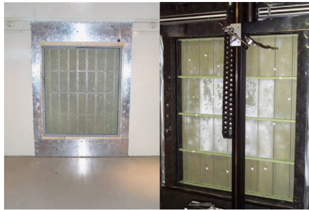
Fig. 12. Pictures of the orthogonally ribbed panel mounted between the reverberant and anechoic rooms; seen from the excitation room (left) and the receiver room (right).
