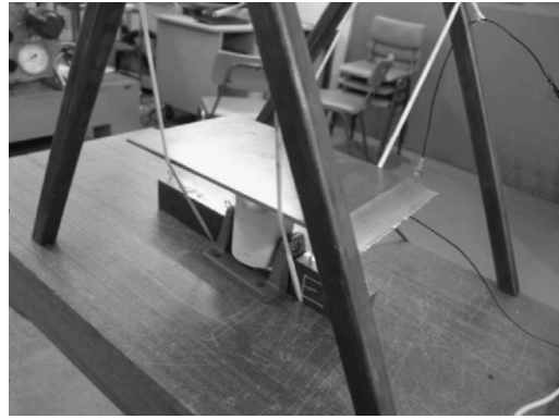
Fig. 7. Experimental apparatus; the plate rests on straps, with the electromagnetic shaker attached to the underside with wax.
