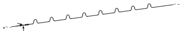
Fig. 14. An infinitely long pipe with the eight ‘periodicity cells’ inserted; pipe diameter 30 mm and wall thickness 2 mm, \rho_s=7800 \text{ kg/m}^3 , \rho_f=1000 \text{ kg/m}^3 , E=210 \text{ GPa} and \nu=0.3 . The wavy arrows designate infinitely long segments.
