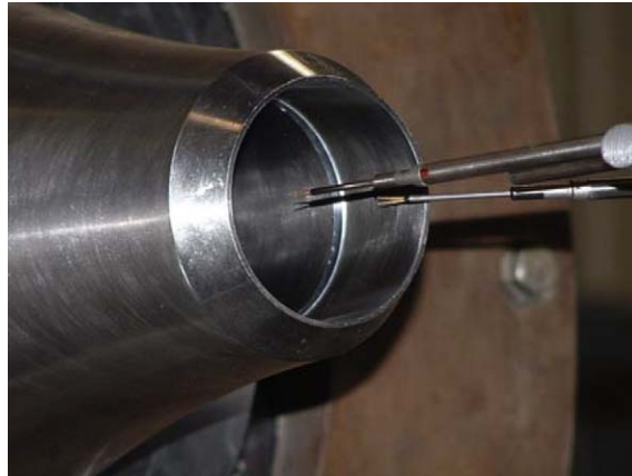
Fig. 2. Photograph of nozzle with two hot-wire probes placed near the exit. The trip ring inside the nozzle is visible.
