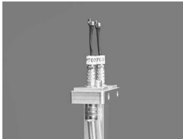
Fig. 1. The special mount with the pair of match size axial sound intensity probes: during the measurement the two probes are aligned along any coordinate axis. Note the anemometric bridge of the two velocity sensors.
