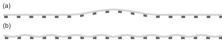
Fig. 11. Mode shapes of the railway track. (a) The P2 mode, where rails and sleepers are bouncing on ballast stiffness. (b) The pinned–pinned mode, which is a bending mode of the rail with the sleepers giving rise to nodes and the sleeper spacing corresponding to half a wavelength.
