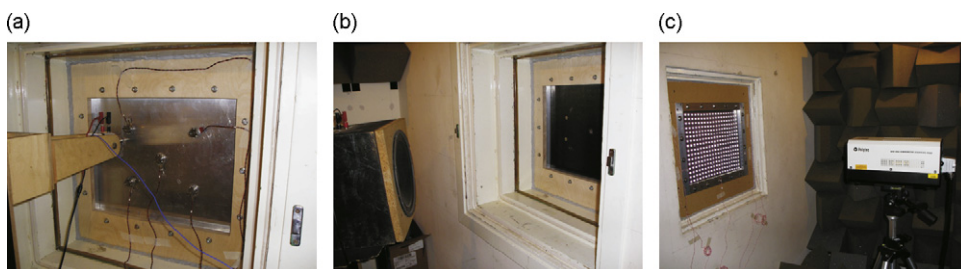
Fig. 14. Set-ups for shaker excitation (a), loudspeaker excitation (b) and laser vibrometer measurements (c).
