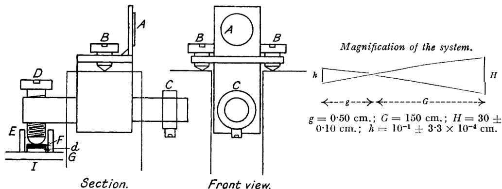
The apparatus consists essentially of an optical lever balanced on a pivot *B* by means of the adjustable counterweight *C*. The end of the screw *D* at the other end of the optical lever just touches a thin brass disc *F*, which rests lightly on a disc of gelatin *d* punched out with a steel punch from Eastman Kodak gelatin.
