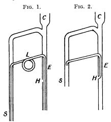
ordinary laboratory apparatus and used for extracting various quantities of material at any temperature above or below that of the room. Ordinary corks used in the apparatus do not come in contact with the liquid solvent, for air is trapped in the extraction flask when it is nearly full (hole H, see below). The construction is simple, strong, and permits of easy repair.
