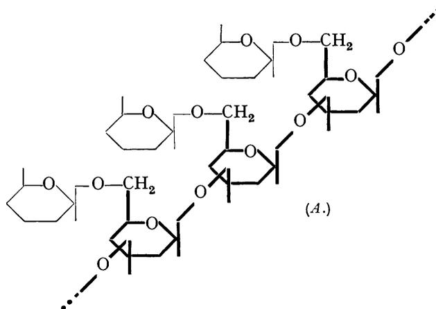
*d*-galactopyranose units linked 1:3 (probably in the  $\beta$ -configuration in view of the change of rotation observed on acid hydrolysis), each unit bearing as side chain a single *d*-galactopyranose unit, glycosidically linked at C<sub>6</sub>; (B) a chain of *d*-galactopyranose units united 1:6, with the side chains attached at C<sub>3</sub>. Both these formulæ admit of an "end
