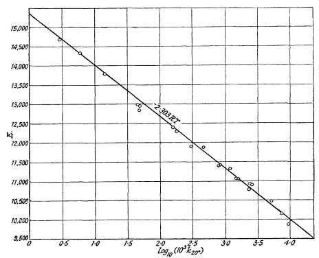
each ether is plotted against E all the points fall on or very near to a line of slope -2.303RT, the intercept of which on the  $\log k$  axis when E=0 gives a value for  $\log PZ$  of 8.46. This result confirms the original conclusion set out above.
