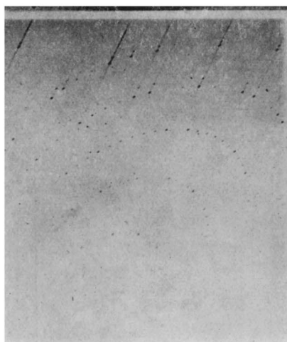
Part of Weissenberg photograph of picryl iodide. Reflexions extending to high values of \theta .
