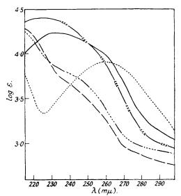
and the original is not available to us. Kortim (Z. physikal. Chem., 1939, B, 42, 39) shows graphically, for nitrobenzene and m-dinitrobenzene in water and s-trinitrobenzene in  $10^{-8}$ N-hydrochloric acid, absorptions at ca. 270 m $\mu$ . (log  $\varepsilon$ , 3.9), ca. 220 m $\mu$ . (log  $\varepsilon$ , 4.2), and below 230 m $\mu$ . (log  $\varepsilon$ , above 4.4), respectively. His results and ours, therefore, despite the change of solvent, are not very dissimilar.
