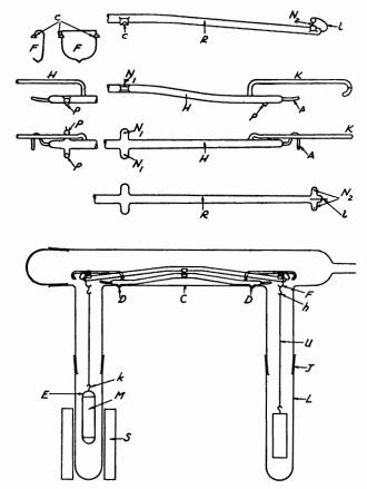
in general varies by only one per cent. or so over a period of months, but should be checked at frequent intervals. The total load on each side of the balance can be 50 g. or more, so that the weight of the working substance may be as high as 25 g. or so if necessary.
