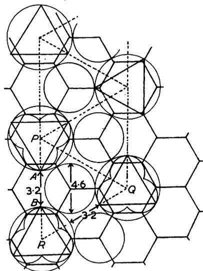
FIG. 9b. Interlamellar orientation suggested for benzene molecules between tetrahedral  $\text{NMe}_4^+$  ions.
