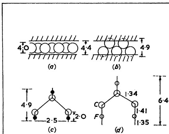
(a) and (b) The flat and vertical orientations of the zig-zag of n-alkane chains in relation to the free distance between sheets in  $\text{NMe}_4$ -montmorillonite.
