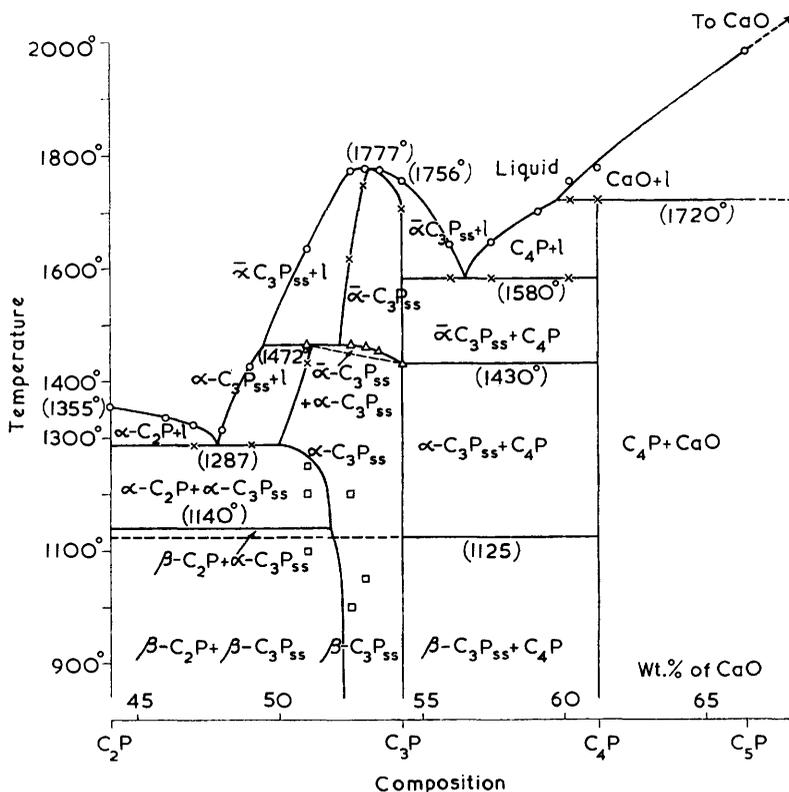
The system  $2\text{CaO}, \text{P}_2\text{O}_5\text{-CaO}$ .
