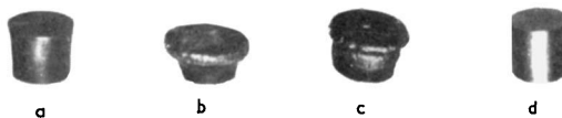
PLATE 6. Projectiles: (a) not detonated; (b) detonation, axial initiation; (c) detonation, non-axial initiation; (d) unfired.
