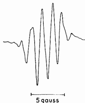
FIG. 7. Derivative electron spin resonance spectrum of the free-radical produced by electrolysis of diquinone (II) in dimethyl sulphoxide.
