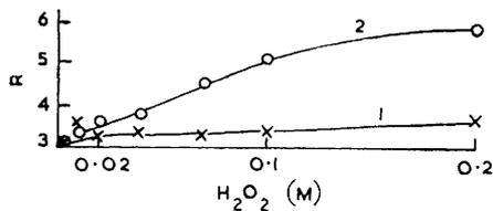
FIG. 5. Photodecomposition of hydrogen peroxide in the presence of saturated benzene solutions as a function of hydrogen peroxide concentration.  $\lambda > 290$  m $\mu$ . The dose absorbed by the same volume of an actinometry solution of uranyl oxalate was  $3.50 \times 10^{-5}$  einstein.
