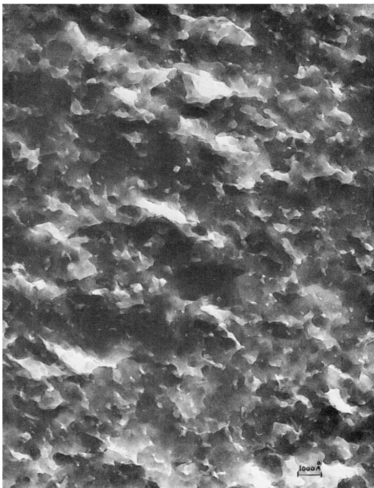
21% Divinylbenzene copolymer ( F_M = 0.6 ) \times 65,000. Corresponding micrographs of linear polystyrene and of conventional 15 and 55% divinylbenzene copolymers were completely featureless.
