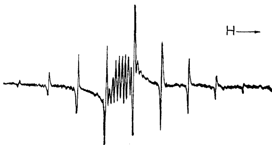
FIG. 3. The spectrum assigned to durene cations, formed by exposure of a dilute solution of durene in oleum to ultraviolet light.
