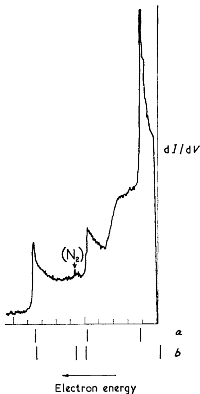
FIGURE 2. Above; the photoelectron spectrum for nitrous oxide ( p = 0.028 mm) to the same electron energy scale as Figure 1
