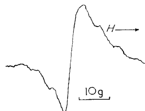
FIGURE 2. Q -Band electron spin resonance spectrum of \text{C}_2(\text{CN})_4^-
