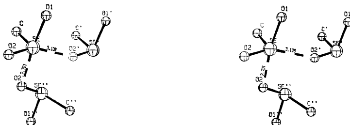
FIGURE 5 Stereoscopic drawing of the environment of the selenium atom in trans -ethanediseleninic anhydride (X) (co-ordinates from ref. 19). The approximately trigonal bipyramidal arrangement of five atoms around the nearest selenium atom can be seen
