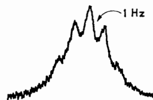
FIGURE 4 The formyl proton resonance of the O -protonated cation of NN -dimethylformamide in 60% perchloric acid at 27 °C and 90 MHz
