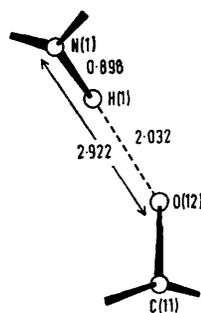
FIGURE 5 Detail of the hydrogen bonding. Distances in Å; angles (deg.): N(1)-H(1)-O(12) 70.7 (38)°, N(1)-O(12)-C(11) 129.6(3)°, and H(1)-O(12)-C(11) 126.7(27)°
