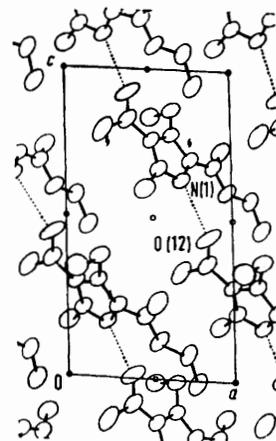
FIGURE 4 A view of the molecular packing, projected along the *b* axis direction. Dashed lines represent hydrogen bonds. N(1) and O(12) are related by the symmetry operation  $(\frac{1}{2} + x, \frac{1}{2} - y, z - \frac{1}{2})$
