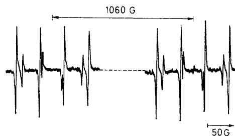
E.s.r. spectrum at 9.130 GHz produced by photolysis of di-t-butyl peroxide in the presence of diethyl chlorophosphite in cyclopropane at -60^\circ
