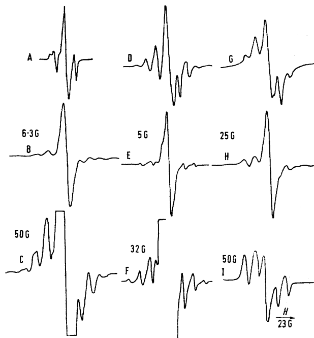
E.s.r. spectra of polycrystalline acyl chlorides recorded at 89 K after \gamma -irradiation at 77 K: A, acetyl chloride; B, C, valeryl chloride at different gains; D, isobutyryl chloride; E, palmitoyl chloride; F, palmitoyl chloride after annealing for ca. 11 h at 262 K; G, methacryloyl chloride; H, I, pivaloyl chloride at different gains
