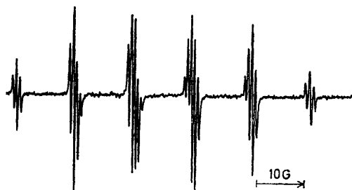
FIGURE 1 A typical spectrum of the nitroxide obtained by radical trapping with 2,4,6-tri- t -butylnitrosobenzene. This spectrum shows the adduct of methyl radical (5) generated by the reaction of methyl iodide with tri- n -butylstannane in benzene at room temperature. The smallest couplings are assigned to the two meta -hydrogens
