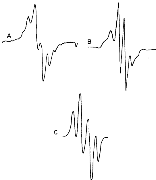
FIGURE 4 E.s.r. spectra of the thiourea adduct of NMCM \gamma -irradiated at 77 K; A recorded at 89 K; B recorded at 298 K; C computer simulation by using a_{2\cdot H} = a_{4\cdot H} = 14 , a_{3\cdot H} = 3 , and a_{5\cdot H} = 21 G
