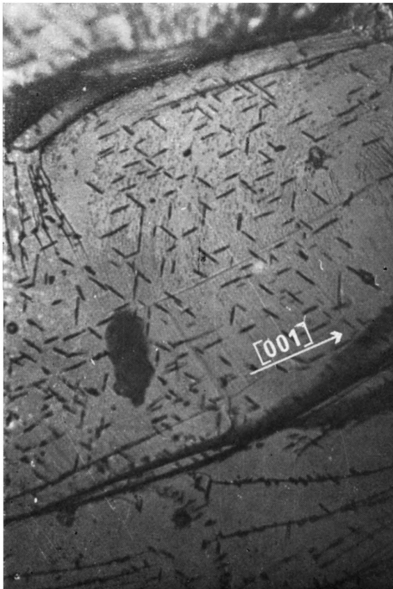
PLATE 4 Typical high-resolution optical micrograph showing nature of orientational relationship between, and alignments of dimer nuclei, at the parent (010) monomer surface (magnification \times 333 )
