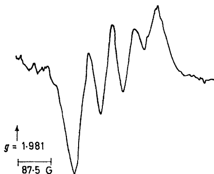
FIGURE 1 E.s.r. spectrum of the Ullmann condensation system [(I)]_0 = 1.25 \times 10^{-2}M , [PhNH_2]_0 = 0.30M , [Cu^{2+}]_0 = 2.5 \times 10^{-4}M , pH = 9.94 , 1a temp. = 20^\circ C
