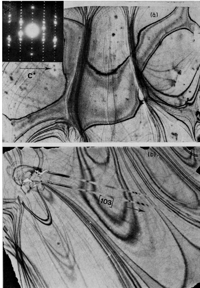
PLATE 3 (a) Typical electron micrograph, with associated diffraction pattern the symmetry and spacing of which shows that the zone axis is [010] , of 1,8-Cl 2 -10MA; no dislocations are visible and the dark lines are bend extinction contours (magnification \times 9000 ). (b) Another micrograph showing striations running closely parallel to [301] directions and signifying existence of planar faults separating two distinct crystallographic phases (see text) (magnification \times 11,000 )
