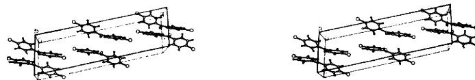
FIGURE 4 Stereoview of the packing of DBP in the unit cell, viewed perpendicular to b
