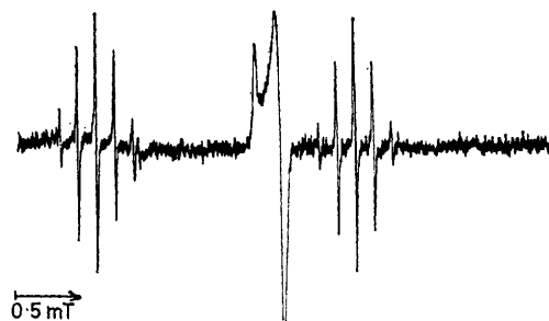
FIGURE 1 E.s.r. spectrum of 1,3-dioxolan-2-yl at -127 °C; the asymmetric resonance is from a paramagnetic impurity in the cell
