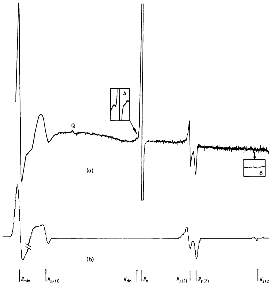
(a) E.s.r. spectrum of p\text{-NH}_2\text{C}_6\text{H}_4^+ in LiCl glass at 77 K. H_o , radical absorption of p\text{-NH}_2\text{C}_6\text{H}_4^+ ; inserts A, B, regions of H_{dq} and H_{z(2)} absorption; Q, quartz signal. (b) Computer simulation of (a) based on 20 000 orientations with accuracy \pm 0.9\text{ mT}
