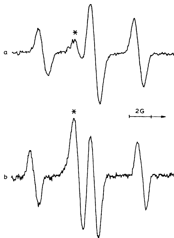
FIGURE 2 Lines 4--6 of the e.s.r. spectra of (1; \text{R} = \text{Me} or \text{Bu}^t ) and (marked *) line 2 of \text{Me}\cdot or line 5 of \text{Bu}^t\cdot at 233 K. a, \text{R} = \text{Bu}^t , cyclopentane solvent, [\text{DEVP}] 0.16, [(1; \text{R} = \text{Bu}^t)] 1.2 \times 10^{-6} , [\text{Bu}^t\cdot] 1.3 \times 10^{-7}\text{M} ; b, \text{R} = \text{Me} , cyclopropane solvent, [\text{DEVP}] 0.63, [(1; \text{R} = \text{Me})] 3.8 \times 10^{-7} , [\text{Me}\cdot] 2.0 \times 10^{-7}\text{M}
