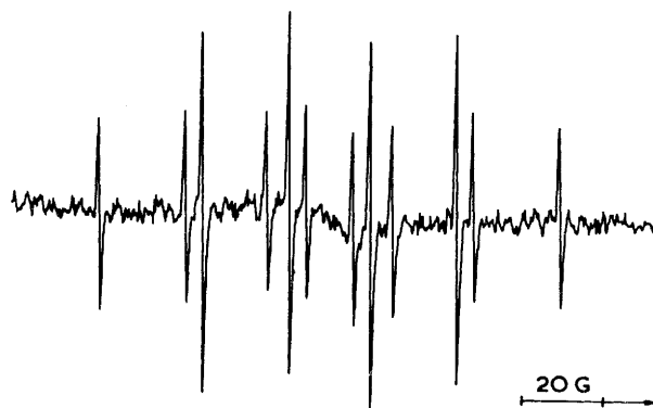
FIGURE 3 E.s.r. spectrum of (1; \text{R} = \text{Me} ) obtained during photolysis of a cyclopropane solution containing diethyl 1-bromopropylphosphonate, di- t -butyl peroxide, and triethylsilane at 235 K
