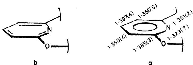
FIGURE 6 a, Average bond distances for the asymmetrically disubstituted pyridine rings of both molecules. b, Bonding representation for the asymmetrically disubstituted pyridine rings
